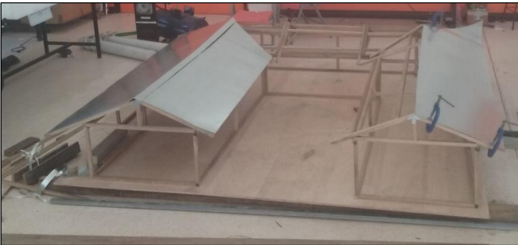
Figure 15: Installation of ridge caps and V-drains.
