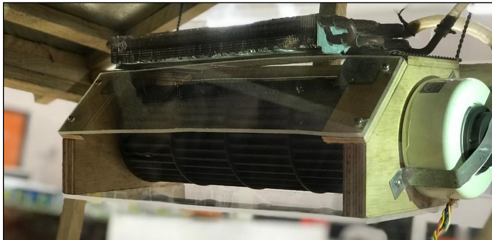
Figure 18: Final assembled AHU.
