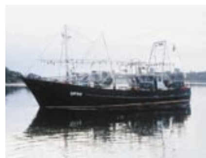
Figure 3-9 Combined squid-jig vessel & purse seiner Australia Source: AFMA (2006)
