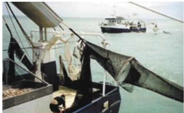
Figure 3-19 Turtle excluder device in trawl net AFFA (2006)
