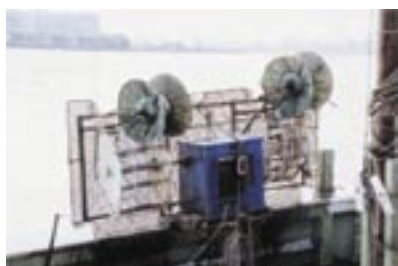
Figure 3-17 Automatic Squid jigging machine
